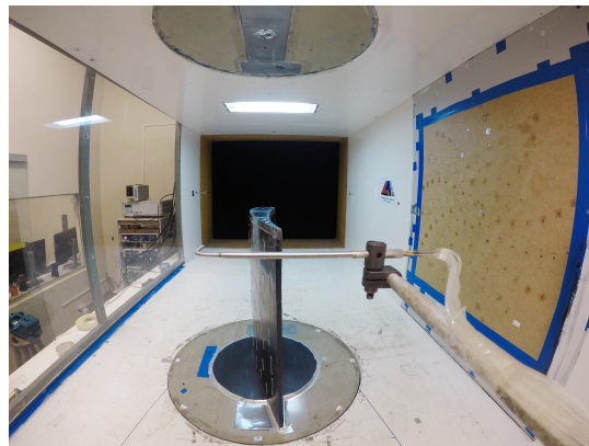
Fig. 14 7-hold pitot probe behind the flap model.
